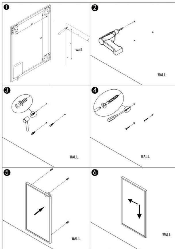
Step 1. Measure the distance between the mounting hooks and mark the position on the wall.
