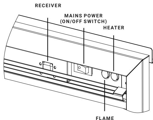
**NOTE:** The flame is always on when the unit is switched on.
